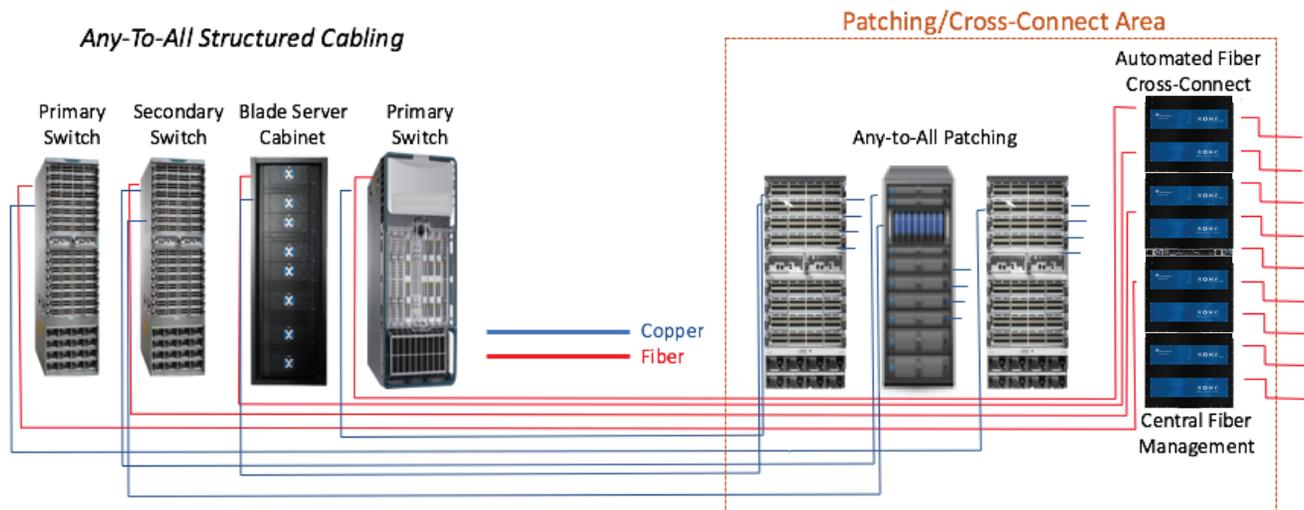
The inherent programmability of SDI ensures that robotic automated cross-connects are dynamic and—unlike physical cross-connects or switches—device connections can be modified quickly. A wide variety of use cases—including network monitoring and security applications—are well suited to the robotic cross-connect approach. This functionality is currently available today, from next generation products such as Wave2Wave’s ROME product family.
