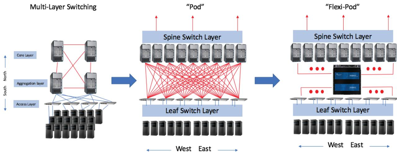
Even without Spine-Leaf architectures, the increasing number of parallel optics that use eight fibers per port instead of the traditional two fibers per port is also creating unprecedented growth in fiber cabling. Therefore, Data Center fiber counts will increase regardless of spine-and-leaf or traditional three-layer architectures, requiring enhanced Layer-0 management capabilities to keep pace with growth.
